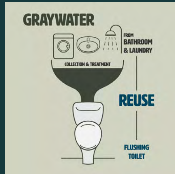
Figure 19. Toilet graywater system
