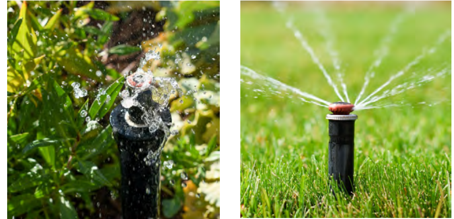
Figure 30. Types of overhead spray irrigation heads: spray head and rotary nozzle
